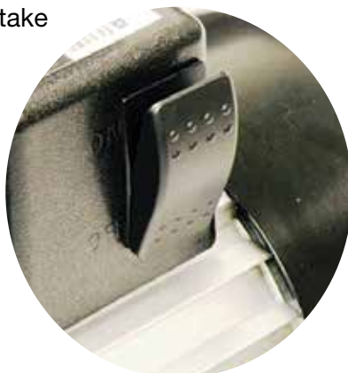
Sealed starting switch on ignition-proof models
